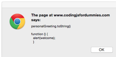
Figure 15-3: A closure includes the code of the returned inner function.
